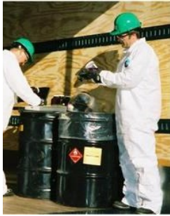
Packaging hazardous waste in a lab pack for off-site transportation and disposal.
