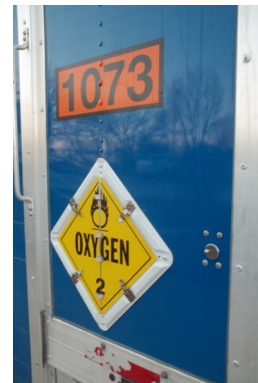
The use of a placard with an orange panel containing the identification number marking.
